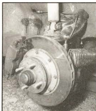
Front suspension fully rose-jointed with AP four pot braking, for tarmac stages . . . . .
