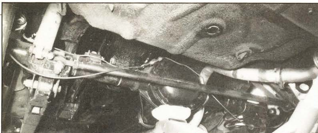
Manta A-Series rear axle mounted using four link bars and a Panhard rod. Turrets hold Bilstein dampers vertical.
