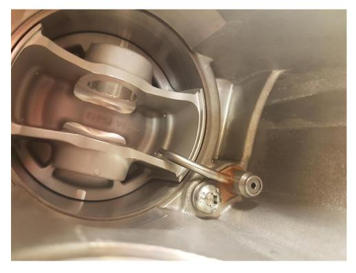
The photo above shows how the oil squirter should be positioned, with it clearing the piston and aimed toward the middle of the piston.
