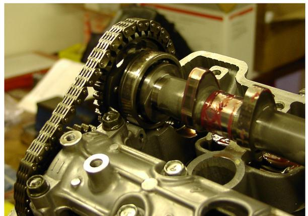
7. Next fit the cam carrier and torque down to the correct setting-note tighten each bolt a little at a time to equalise the pressure over the cam and carrier.
