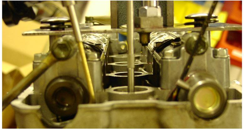
14. Rotate the engine and as the valves close on the followers that you are measuring the DTI's can be zeroed when the cam lobe is completely pointing away from the follower.
