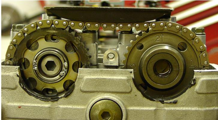
12. The engine can now carefully be rotated in the normal direction (anti-clockwise when viewed from the generator end) at least two complete revolutions. ***Pay particular attention to any resistance felt when rotating the engine encase this is the valves touching the pistons.***
