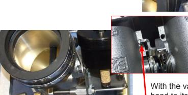
With the vacuum blipper installed, operate the blip by hand to its maximum travel, you must ensure the pin does not fall off the lever arm.
