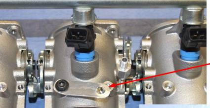
Temporarily fit the supplied stabilising strip to the mounting hole as shown in the picture below, then mark on the strip where you require to drill through in order to bolt to the throttle blip actuator.
